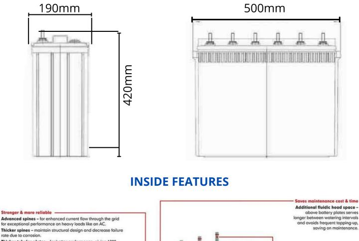
Thicker tubular plates - for better performance, giving 1200 cycles @ 80% depth of discharge.
